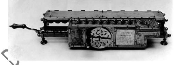
The Step ReckonerA reproduction of Gottfried Wilhelm von Leibniz's Step Reckoner, from the original located in the Trinks Brunsviga Museum at Hannover, Germany. Turning the crank (left) rotated several drums, each of which turned a gear connected to a digital counter. *IBM Archives*
