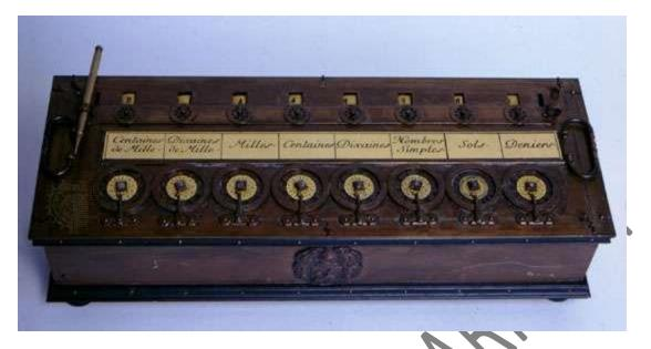
The Arithmetic MachineThe Arithmetic Machine, or Pascaline, a French monetary (nondecimal) calculator designed by Blaise Pascal *c*. 1642. Numbers could be added by turning the wheels (located along the bottom of the machine) clockwise and subtracted by turning the wheels counterclockwise. Each digit in the answer was displayed in a separate window, visible at the top of the photograph. *Courtesy of the Computer Museum History Center*
