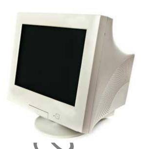
A finite number of characters can be displayed on a screen at once. The screen can be divided into a series of character boxes - fixed location on the screen where a standard character can be placed. Most screens are capable of displaying 80 characters of data horizontally and 25 lines vertically.
